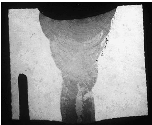
Fig. 1. Metallograph of a re-welded powder hipped stainless steel sample (irradiated material on the right, un-irradiated on the left) showing significant cracking in the HAZ of the irradiated material.
